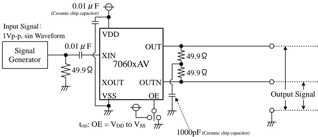
Fig 12-4. Measurement circuit 4
