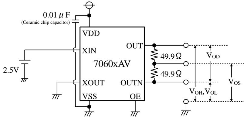
Fig 12-2. Measurement circuit 2
