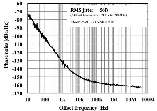
7060EAV,  $f_{OUT}=155.52\text{MHz}$ ,  $V_{DD}=1.8\text{V}$ ,  $T_a=25^\circ\text{C}$
