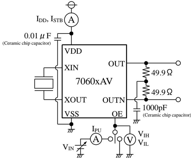
$$R_{PU1} = \frac{V_{DD}}{I_{PU}} \quad (V_{IN} = V_{SS})$$
